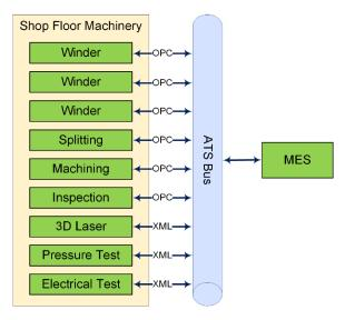
ATS has implemented ATS Bus which is handling production order information being sent from the MES layer down to the machines. The machines in turn send back production data collected during the operation and when it's complete an *Operation Complete* message is sent to MES containing all of the gathered data.
